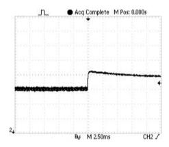
Figure below shows a typical output voltage response, measured during a transition from 20% load current to full rated load current with no additional output filtering.
