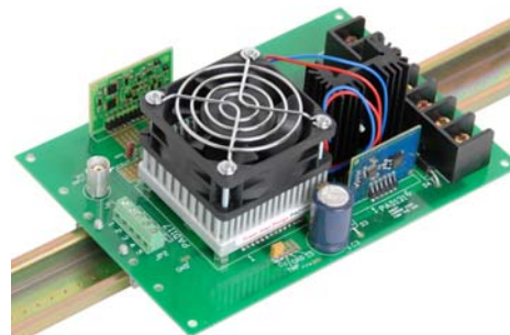
PAD116 MOUNTED IN EVALUATION KIT
