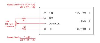
Figure below shows how to remotely mechanically shutdown the converter while maintaining any preset control voltage.
