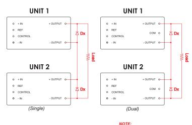
The ratings of Dx should be 1.5 times the maximum current and voltage expected in each branch.
