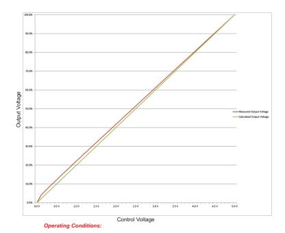
Output Load = Resistive (fixed at full output current @ 100% output voltage)
