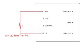
The figure below shows how to combine both of the prior configurations to form upper and lower boundaries for the adjustable range.
