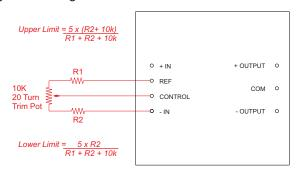
Figure below shows how to remotely mechanically shutdown the converter while maintaining any preset control voltage.
