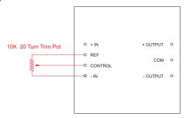
The figure below shows how to combine both of the prior configurations to form upper and lower boundaries for the adjustable range.
