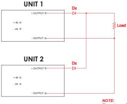
The ratings of Dx should be 1.5 times the maximum current and voltage expected in each branch.
