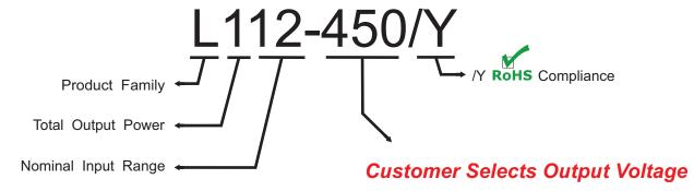
The L1 Series are designed such that the customer may order any output voltage from 24Vdc to 500Vdc at no additional charge.
