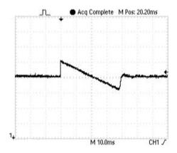
Figure below shows a typical output voltage response, measured during a transition from no load current to full rated load current with no additional output filtering.
