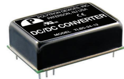
These 5-watt DC-DC converters integrate a six-sided continuous shield and built-in EN55022 Class B filter. Units are housed in an industry-standard DIP package and meet all relevant UL safety standards.
