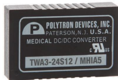
Housed in a miniature DIP package, these 3-watt 2:1 wide input DC-DC converters feature a clearance and creepage distance of 8 mm/2 MOPP and built-in Class A filter.
