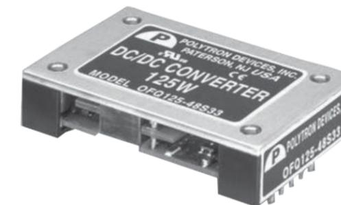
With a single output up to 35 A and no minimum load requirement, these 125-watt quarter-brick DC-DC converters feature an adjustable output voltage, as well as UL and CE safety approvals.
