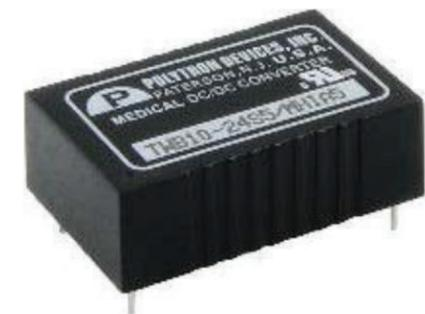
Designed for medical safety and housed in a miniature DIP package, these 10-watt single and dual output DC-DC converters have a patient leakage current of 2  $\mu$ A and clearance and creepage distance of 8 mm/2 MOPP.
