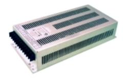
The LIN 67 Series of AC/DC converters uses high frequency dual FET forward topology to generate 100W output power. Virtually any DC output is possible with short delivery times. This low profile design features low component count and high efficiency. The use of high quality components and rigorous quality control results in an MTBF exceeding 100,000 hours at 45°C. The LIN67 modules are also available in Eurocard format.
