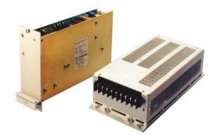
The EOL 76 Series off-line power supply is an advanced, field-proven design utilizing a dual-FET diagonal half-bridge topology. The switching frequency for the standard version is 125kHz. The unit is fully protected and is manufactured using high quality components which contributes to MTBF ratings exceeding 100,000 hours.
