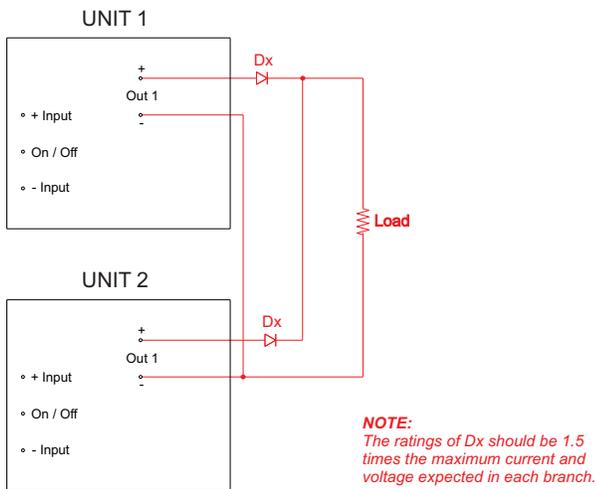
The figure below shows how to connect several dual output units with equal nominal output voltage in parallel.
