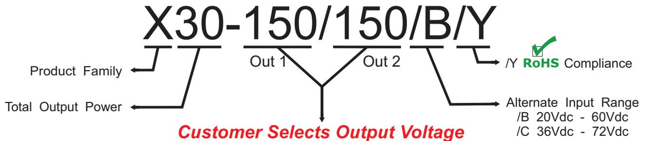
The X30 Series are designed such that the customer may order any output voltage from 24Vdc to 500Vdc at no additional charge.
