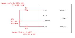
Figure below shows how to remotely mechanically shutdown the converter while maintaining any preset control voltage.
