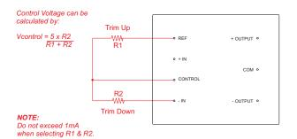
The figure below shows how to adjust the output voltage using an external Trim Pot.
