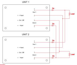
The ratings of Dx should be 1.5 times the maximum current and voltage expected in each branch.
