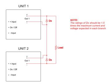
Figure below shows how to connect multiple dual output units in series with the use of shunt diodes.
