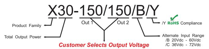
The X30 Series are designed such that the customer may order any output voltage from 24Vdc to 500Vdc at no additional charge.
