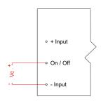
**NOTE:**Do not exceed 6Vdc on remote On/Off. otherwise, the supply may be permanently damaged.
