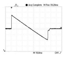
Figure below shows a typical output voltage response, measured during a transition from no load current to full rated load current with no additional output filtering.
