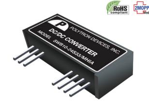
These regulated DC-DC converters provide up to 10 watts of power and efficiency up to 83 percent. Units are suitable for medical applications, as well as industrial and ITE equipment.
