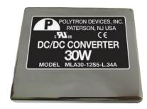
These 30 watt DC-DC converters features high efficiency up to 80 percent, as well as short circuit and over-voltage protection in a low profile  $3.0 \times 2.5 \times 0.3$ " package. Epoxy encapsulated, this series also features ON/OFF control and is RoHS II compliant.
