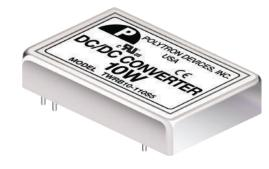
Housed in a miniature DIP package, these 10-watt single and dual output DC-DC converters feature 1,500 VDC isolation voltage, 100 percent burn-in for reliability and remote ON/OFF control for energy savings in railway applications.
