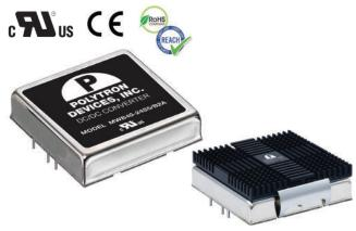
These isolated 40-watt single and dual output DC-DC converters offer high efficiency up to 89 percent, 1,600 VDC isolation and remote ON/OFF control for energy savings. A six-sided continuous shield minimizes noise leakage.
