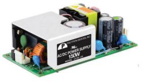
For industrial applications, these 150-watt AC-DC converters provide high efficiency up to 92 percent and include low leakage current and standby power for additional energy savings.
