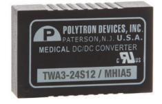
Housed in a miniature DIP package, these 3-watt 2:1 wide input DC-DC converters feature a clearance and creepage distance of 8 mm/2 MOPP and built-in Class A filter.
