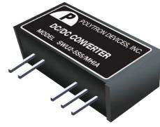
Designed for medical applications, this series of 2-watt single and dual output DC-DC converters has a patient leakage current rating of 2 µA and is housed in an industry-standard 7-pin SIP package.
