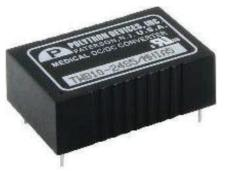
Designed for medical safety and housed in a miniature DIP package, these 10-watt single and dual output DC-DC converters have a patient leakage current of 2 µA and clearance and creepage distance of 8 mm/2 MOPP.
