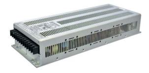
The LVC319 Series AC/DC power supply uses an advanced high frequency conversion technology to generate 500W output power at 12VDC with convection cooling. This low profile design features low component count and high efficiency. The use of professional quality components and rigorous quality control results in an MTBF exceeding 100,000 hours at 45°C.
