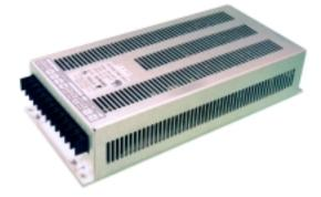
The FOW236 Series of DC/DC converters uses high frequency push-pull forward topology to generate 150W of output power. Virtually any DC output is possible with short delivery times. This low profile design features low component count and high efficiency. The use of high quality components and rigorous quality control results in an MTBF exceeding 100,000 hours at 45°C.
