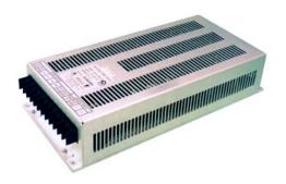
The EOL95 Series of AC/DC converters uses high frequency dual FET forward topology to generate 180W of output power. Virtually any DC output is possible with short delivery times. This low profile design features low component count and high efficiency. The use of high quality components and rigorous quality control results in an MTBF exceeding 100,000 hours at 45°C.
