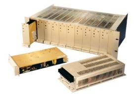
The EOL 67 Series of AC/DC converters uses high frequency forward topology to generate up to 150W output power per plug-in module. Virtually any DC output is possible with short delivery times. This low profile design features low component count and high efficiency. The use of high quality components and rigorous quality control results in an MTBF exceeding 100,000 hours at 45 °C. The EOL67 modules can be parallel-connected for greater output power and/or to achieve N+1 redundancy.
