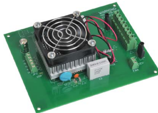
Assembled EVAL189 with amplifier installed.
