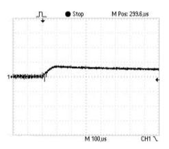
Figure below shows a typical output voltage response, measured during a transition from 20% load current to full rated load current with no additional output filtering.
