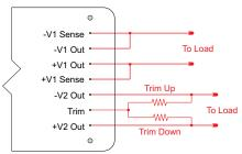
The figures below show how to adjust the output voltage using an external Trim Pot.
