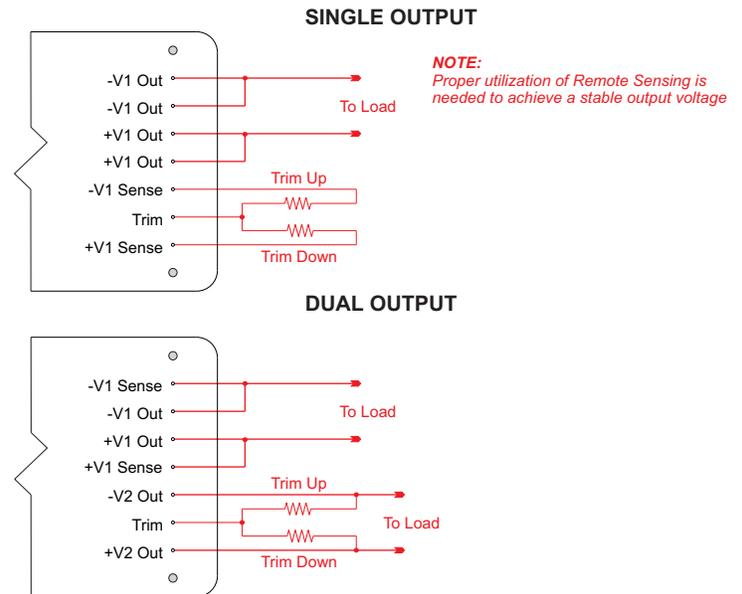
The figures below show how to adjust the output voltage using an external Trim Pot.
