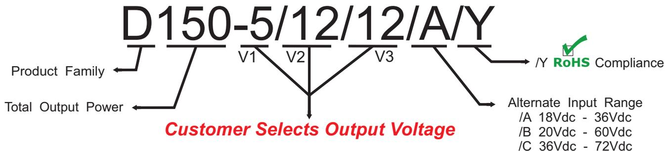
The D150 Series are designed such that the customer may order any output voltage combination from 5Vdc to 28Vdc at no additional charge.
