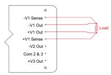
If remote sensing is not required, the SENSE(-) pin must be connected to the Output(-) pin and the SENSE(+) pin must be connected to the Output(+) pin to ensure the converter will regulate at the specified output voltage. If these connections are not made, the converter will deliver an output voltage that is slightly higher than the specified value.
