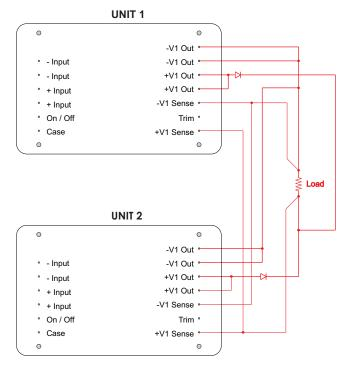
**NOTE:**Current sharing can be adjusted by trimming both converters to the same output voltage
