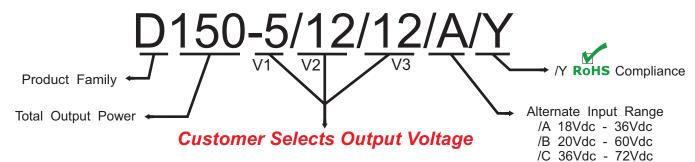
The D150 Series are designed such that the customer may order any output voltage combination from 5Vdc to 28Vdc at no additional charge.
