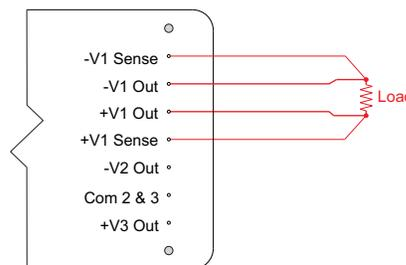
If remote sensing is not required, the SENSE(-) pin must be connected to the Output(-) pin and the SENSE(+) pin must be connected to the Output(+) pin to ensure the converter will regulate at the specified output voltage. If these connections are not made, the converter will deliver an output voltage that is slightly higher than the specified value.
